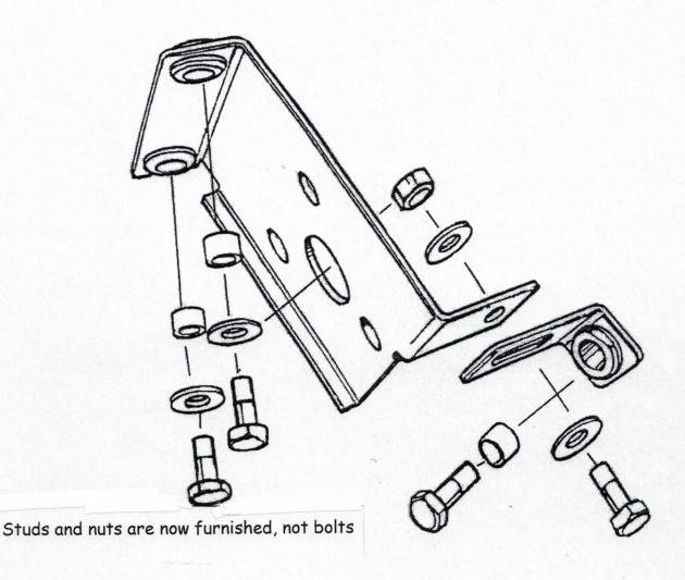
Motor Mounting Bracket (motor not shown)
