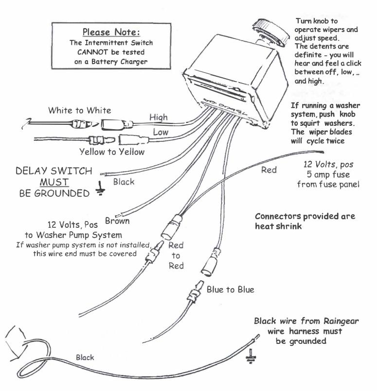
**NOTE:** The colors of the wires from the wiper motor and the colors of the wires on the harness do not match. This is correct.
